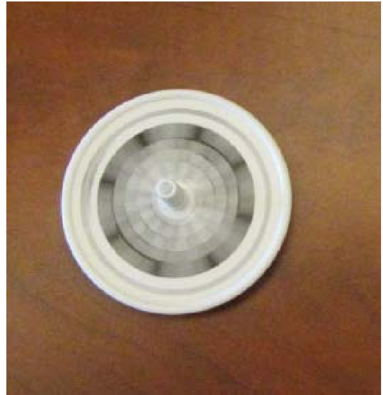
Flicker top showing stroboscopic effect from OLED lighting installation Photo: Aurora Lighting Design, Inc.
