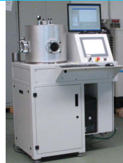
Argonne's sealed methane tribometer
