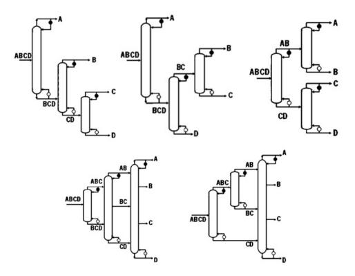
Systematic and easy-to-use method to generate complete set of basic distillation configurations<sup>1</sup>
