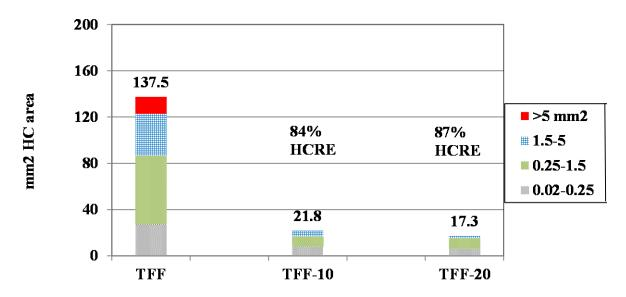
HC: Hydrophobic Contaminants; TFF: Tertiary Fine Screen Feed; HCRE: Hydrophobic Contaminant Removal Efficiency TFF-10 and TFF-20 correspond to 10 and 20 minutes duration in BNF.
