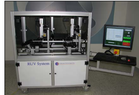
RUV system for in-line crack detection
