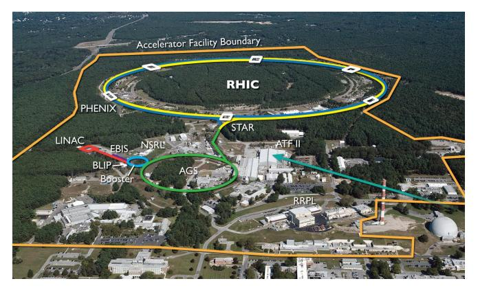
Figure 3: Collider Accelerator Complex Boundaries.
