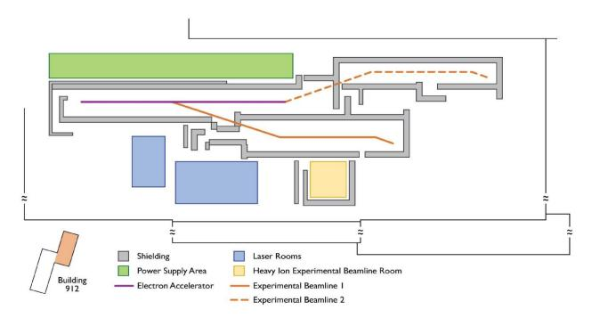
Figure 5: Plan View of ATF Upgrade to 10 GeV in
