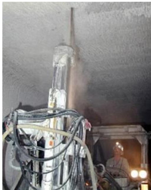
Figure 24: Roof Bolter Drilling to Install Roof Bolts
