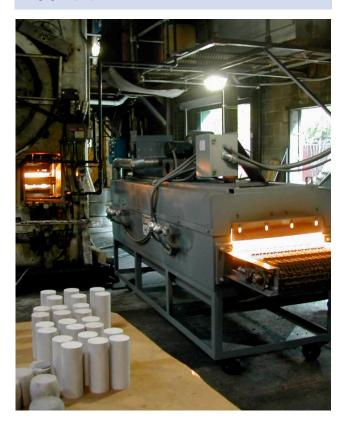
efficient than conventional ovens, and the system proved robust under industrial conditions. The IR furnace demonstrated a downtime of less than 5% over three years of use in preheating billets.
