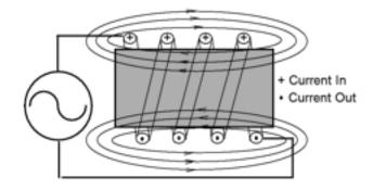
Figure 6.1.6 Schematic of Industrial Induction Heating System. Energy is introduced via inductive coupling between a coil applicator and the product.
