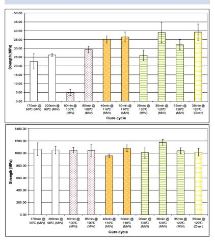
(perpendicular to fibers) and 0° (parallel to fibers) tensile tests. The right-most yellow bar shows the results of the oven-cured sample, and the other bars show the results from the VHM system for various cure cycles, demonstrating statistically comparable performance.<sup>97</sup>
