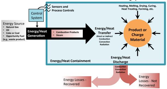
**Combustion-based Process Heating System**
