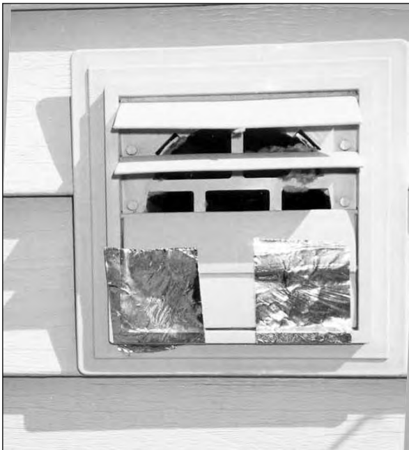
By taping shut first, two, and then, three louvers on the vent hood, I raised static pressures in the venting system.
