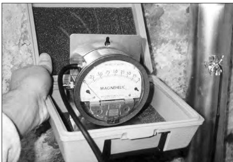
(left) If space is tight between the dryer and the wall, a periscope vent allows the dryer to be 2 inches closer to the wall. (right) I stuck this gauge's right-angled terminal tube into a vertical section of the vent to measure static pressure.
