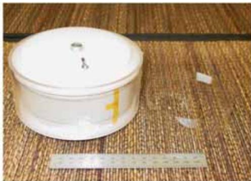
Coiled glass capacitor fabricated at Penn State by spraying Ag ink on the glass ribbon and then winding the ribbon around a mullite mandrel.
