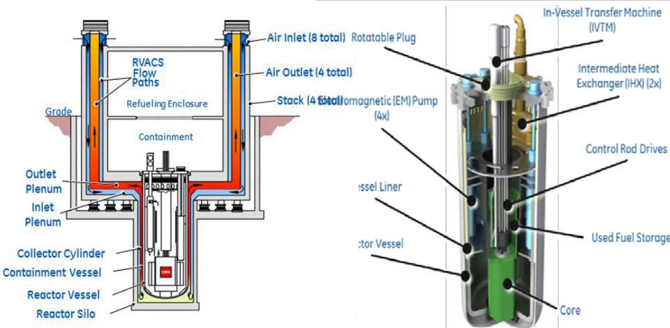
Strategic Objective 4: Test Reactor to Provide Fast Neutrons – Sodium-cooled Fast Test Reactor
