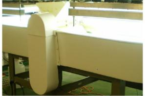
Environmental Simulated Culture Ponds allow full control over solar radiance and water temperature to mimic conditions at different times, seasons and locations.
