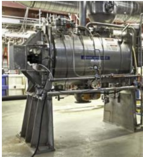
2000 L Deacetylation/Impregnation Mix Tank
