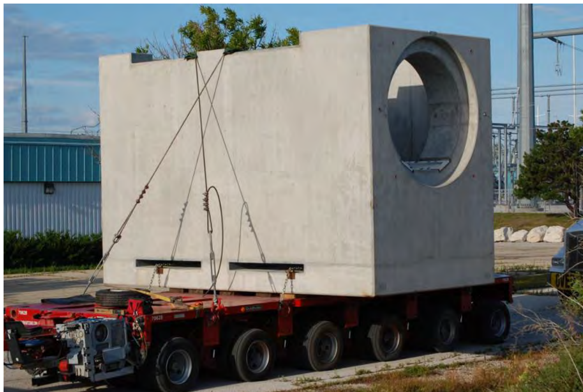
Figure 2-244. Horizontal Storage Module on 6-axle Goldhofer Trailer (2013)
