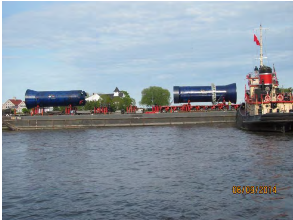
Figure 2-247. Barge with Two Steam Generators at Kewaunee Barge Transload Location (2014)
