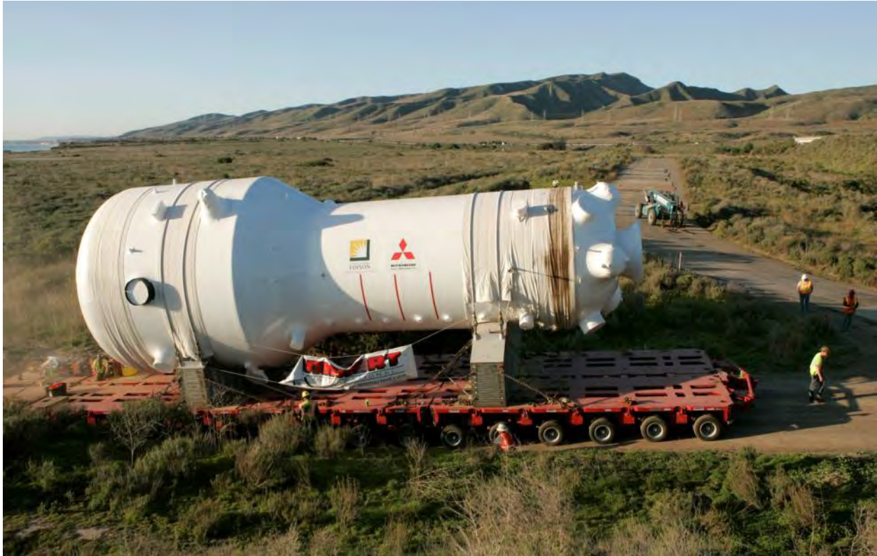
Figure 2-286. Steam Generator on Goldhofer Trailer (2009)
