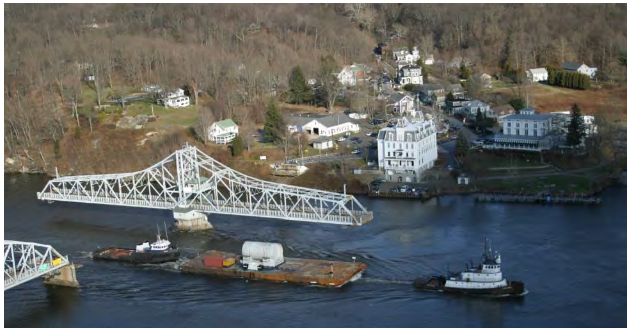
Figure 2-40. Connecticut Yankee Reactor Pressure Vessel Being Transported on Barge in the Connecticut River
