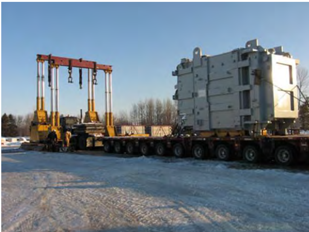
Figure 2-206. Gantry System Used to Transfer Transformers from Railcars to Goldhofer Trailers (2008)
