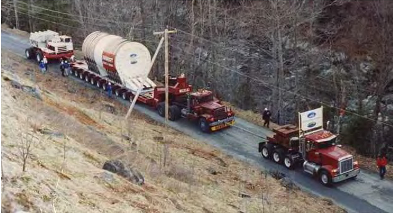
Figure 2-24. Yankee Rowe Reactor Pressure Vessel on Heavy Haul Truck (1997)
