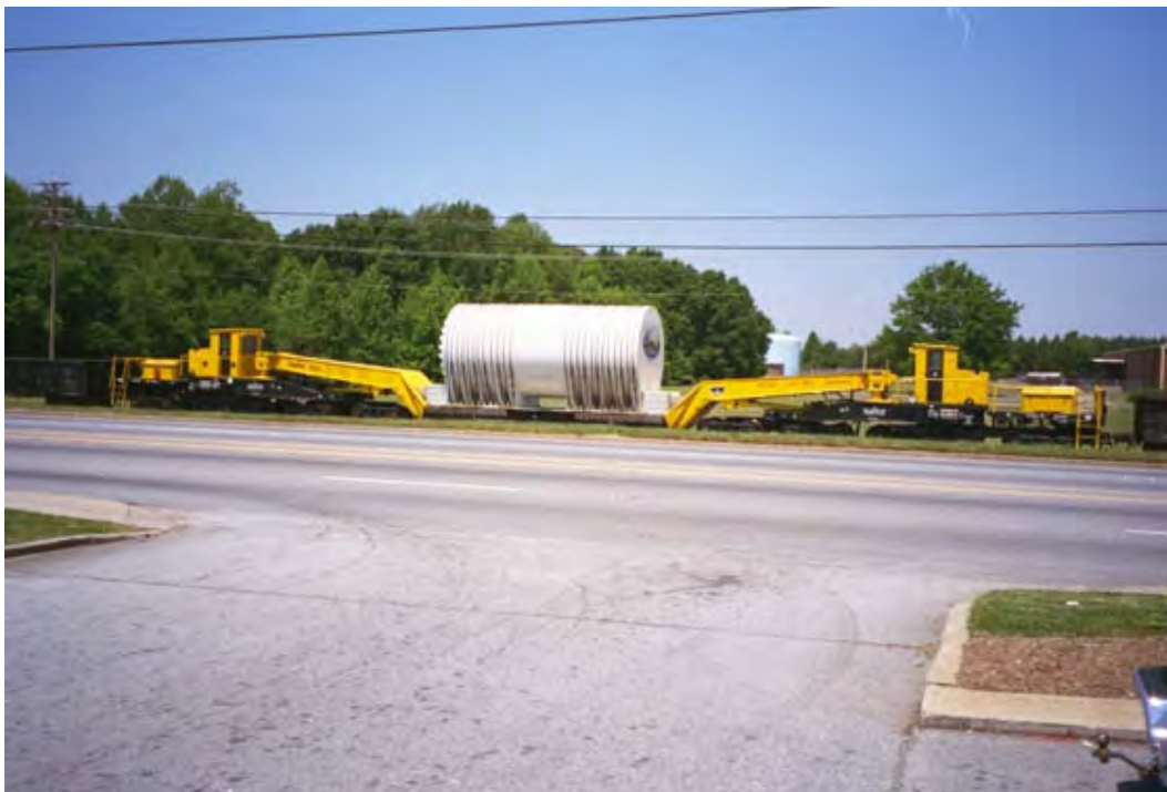
Figure 2-27. Yankee Rowe Reactor Pressure Vessel on Railcar (1997)
