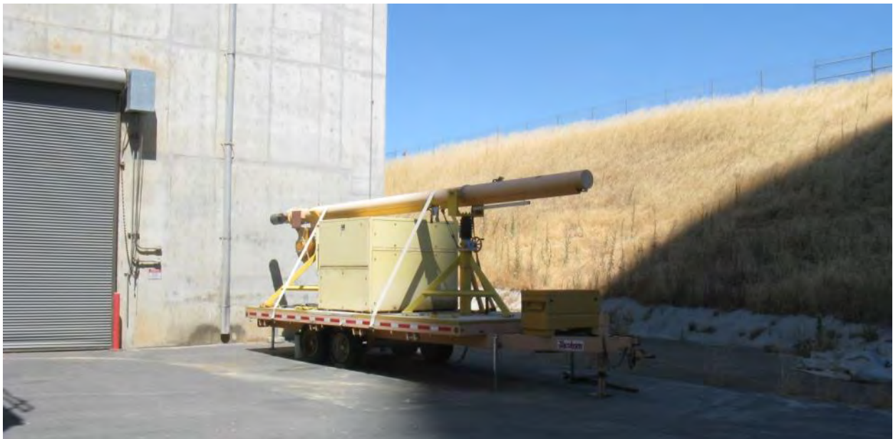
Figure 2-82. Hydraulic Ram Used to Emplace and Withdraw Canisters from Horizontal Storage Modules at Rancho Seco (2013)
