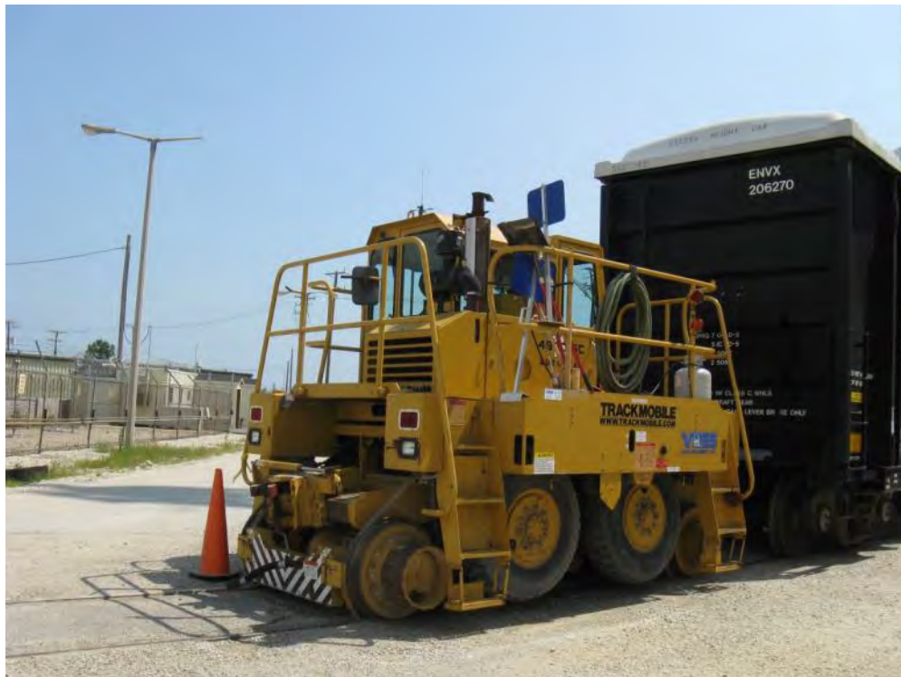
Figure 2-140. Trackmobile Used to Move Railcars On-site (2013)
