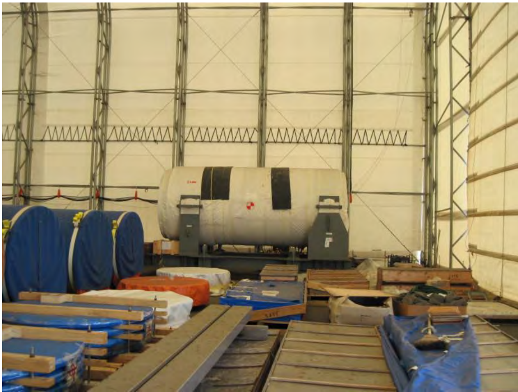
Figure 2-258. Transfer Cask for 32PTH2 Canisters (2015)
