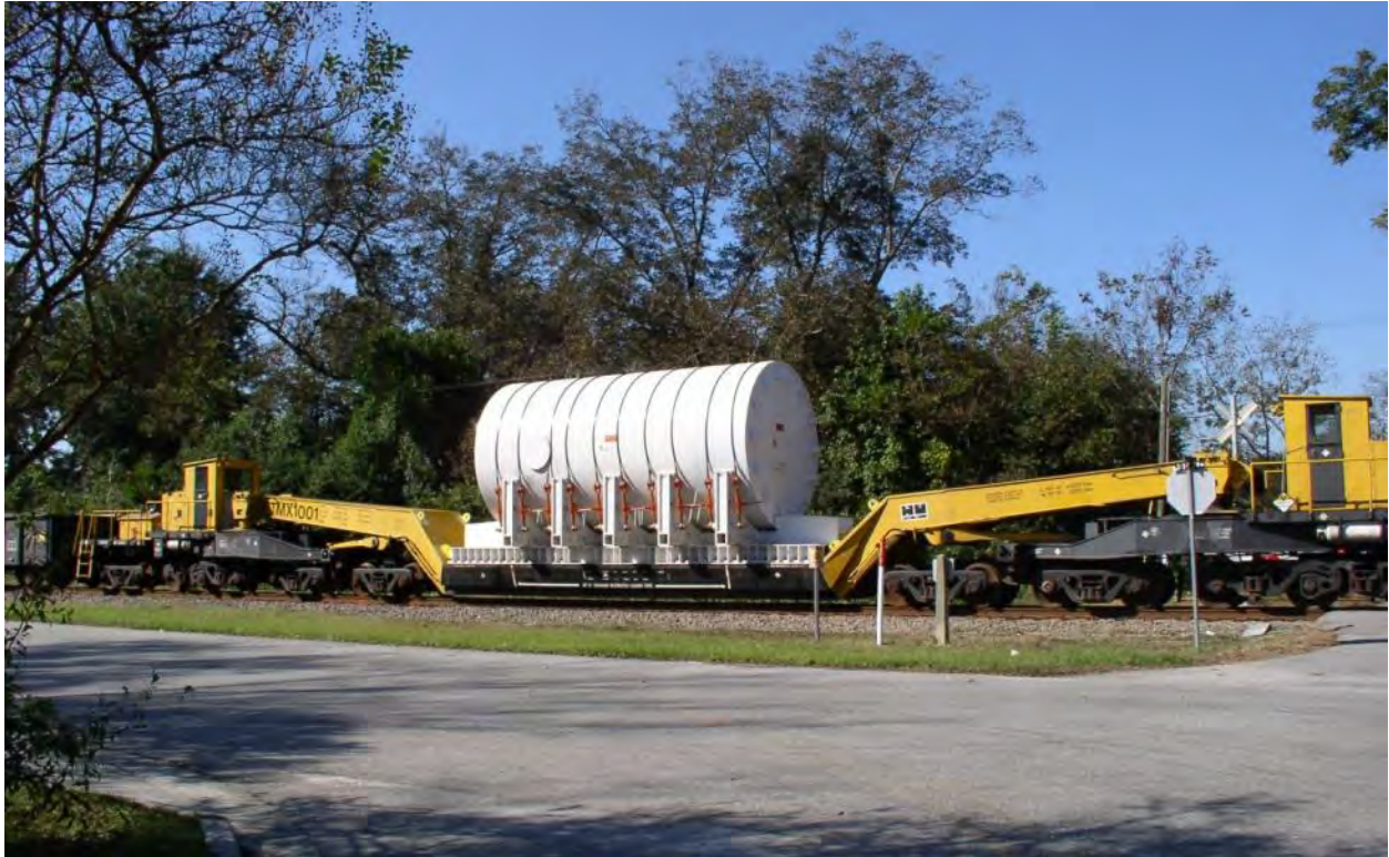
Figure 2-68. Big Rock Point Reactor Pressure Vessel on ETMX1001 Railcar (2003)
