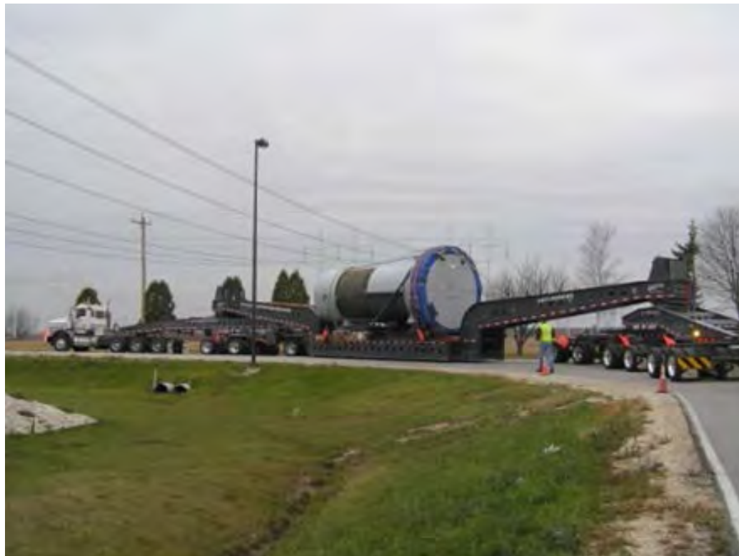
Figure 2-253. Old Reactor Pressure Vessel Head on Heavy Haul Truck (2004)
