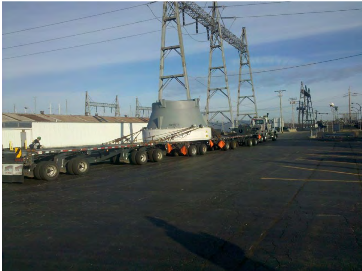
Figure 2-143. Zion Reactor Head on Heavy Haul Truck Transporter (2011)
