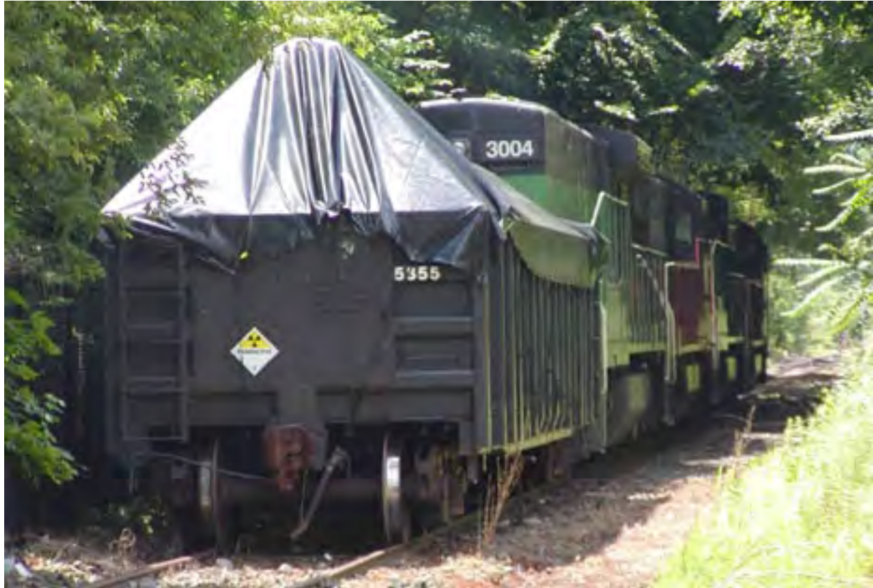
Figure 2-36. Connecticut Yankee Pressurizer at the End of the Portland Rail Spur
