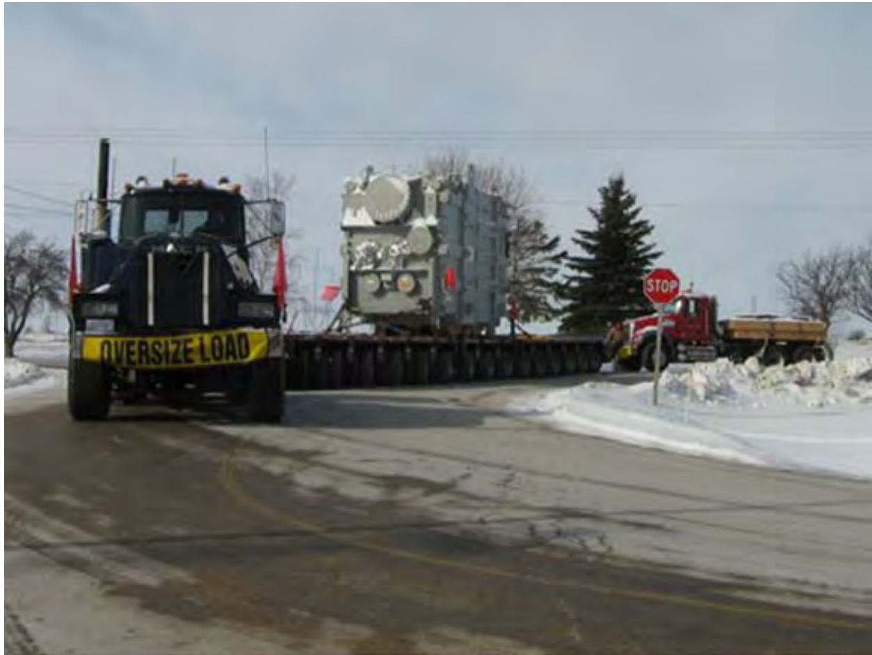
Figure 2-207. Transformer on 15-axle Goldhofer Trailer (2008)
