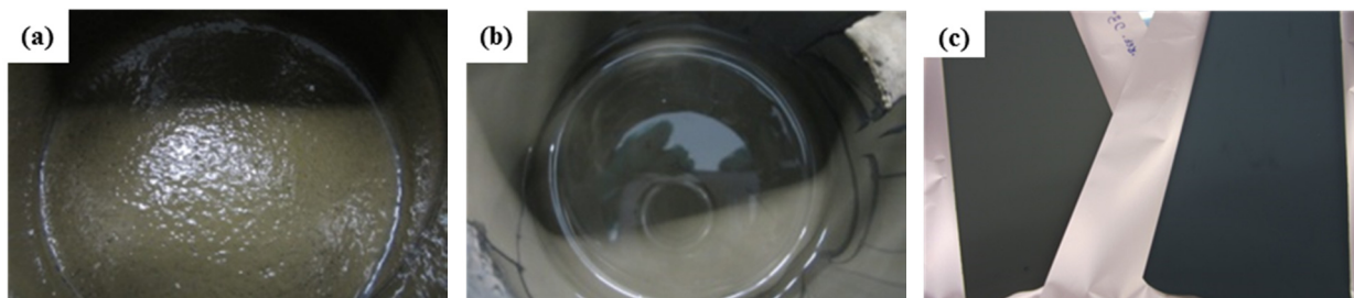
Figure V- 14: Photos of anode slurry (a) nano-Si in \text{H}_2\text{O} with \text{pH}7.5 , (b) nano-Si in \text{H}_2\text{O} with \text{pH} 4 and (c) the electrodes of slurry (a) left and of slurry (b) right
