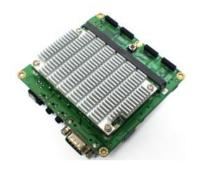
CPU: Arm Cortex A9 Quad core @ 1 GHz RAM: 1 GB Price: \$129 Size: 3.4"x2.4"
