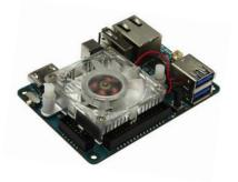
CPU: Arm Cortex A15x4 @2GHz, A7x4 @1.4GHz RAM: 2 GB Price: \$74 Size: 3.3"x2.3" WANDBOARD.ORG
