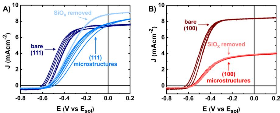
**Figure 30:** Representative illuminated JV curves for **A)** (111) and **B)** (100) microstructures. The (111) microstructures initially out-perform the bare (111) highly-doped substrate, and their performance is improved with removal of  $\text{SiO}_x$ . Conversely, the performance of the (100) microstructures is far below the bare (100) highly doped substrate, and does not improve with etching of the dielectric.
