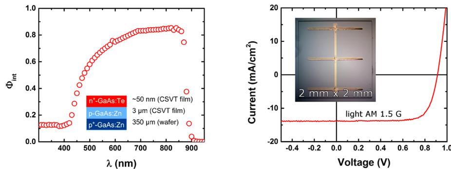
**Figure 15:** Left: JV curve for record efficiency device under 1-sun simulated illumination. Right: Internal quantum efficiency for the same device.
