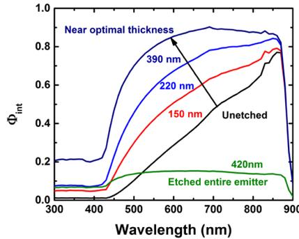
**Figure 11:**  $\Phi_{\text{int}}$  at various etch depths of the device from film 4 with both emitter and absorber grown by CSVT.
