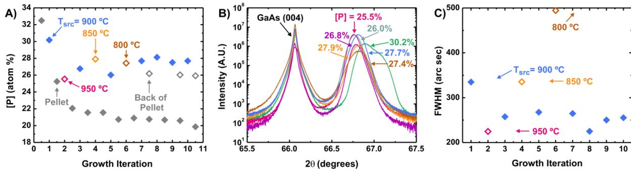
**Figure 20: A)** Evolution of [P] in the  $GaAs_{0.7}P_{0.3}$  source and the resulting varied temperature films. **B)**  $\theta/2\theta$  scans of the first seven varied temperature samples (the others are omitted for clarity). Note the compositional inhomogeneity in sample T1, [P] = 30.2%. **C)** FWHM values from rocking curve scans, which correlate strongly with growth temperature and film thickness. For **A)** and **C)**, films grown at different  $T_{src}$  are indicated.
