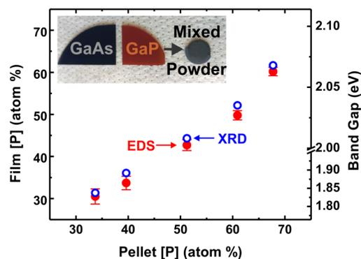
**Figure 18:** The pellet source and film compositions of the varied composition GaAs<sub>1-x</sub>P<sub>x</sub> films. The second y axis shows expected  $E_g$  based on [P]. Images of the source wafers and a pellet are inset.
