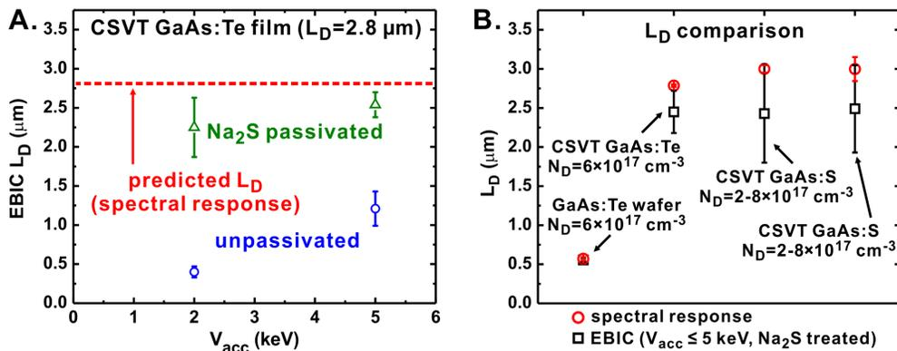
**Figure 7:** (A)  $L_D$  measured by EBIC on the same CSVT GaAs film before and after passivation by  $\text{Na}_2\text{S}$ . The dashed line indicates the  $L_D$  predicted by spectral response. (B) Comparison of  $L_D$  obtained by spectral response and EBIC techniques.
