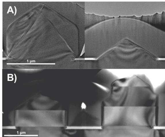
**Figure 29:** Cross-sectional TEM of **A)** (100) and **B)** (111)B GaAs microstructures. Note the stacks of defects present in the larger (100) microstructure which originate at the edge of the  $\text{SiO}_x$  mask, and the single twin plane defects parallel to the growth surface in both (111)B microstructures.
