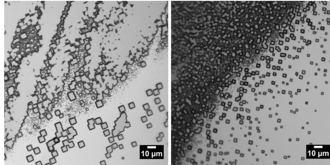
**Figure 32.** Optical microscope images of GaAs grown on a Ge wafer with a substrate temperature of 760 °C. Bare Ge and isolated GaAs islands are visible in the lower right corner, where the film is covered by the quartz spacer during growth. Left: source temperature 800 °C. Right: source temperature 820 °C.
