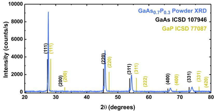
**Figure 21:** Powder XRD scan showing the analyzed pellet (blue) with the literature peak positions for GaAs and GaP shown (black and yellow, respectively) after ten growths. Minor unincorporated regions exist (based on small GaAs peaks in the powder pattern) but the majority of the pellet has been sintered to a ternary phase.
