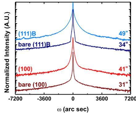
**Figure 28:** High-resolution rocking curves comparing FWHM of the bare commercial (100) and (111)B substrates to those of the microstructured (100) and (111)B samples.
