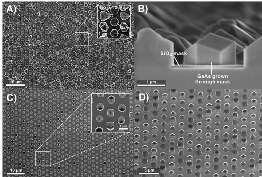
**Figure 27:** SEMs of microstructure growth. **A)** Plan-view and **B)** cross-section of (111)B microstructures with optimized growth conditions  $T_{\text{src}} = 850\text{ }^\circ\text{C}$ ,  $\Delta T = 10\text{ }^\circ\text{C}$  for 10 min,  $50\text{ }^\circ\text{C}$  for 90 s **C)** Plan-view and **D)**  $45^\circ$  tilt of (100) microstructures with optimized growth conditions  $T_{\text{src}} = 850\text{ }^\circ\text{C}$ ,  $\Delta T = 30\text{ }^\circ\text{C}$  for 10 min
