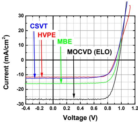
**Figure 16:** IV comparison of devices chosen for TPC/TPI study.
