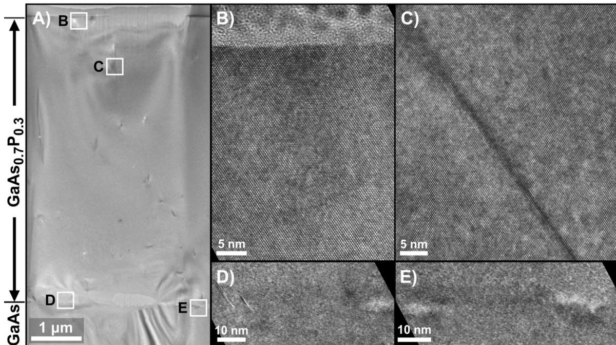
**Figure 23:** TEM of sample T10 FIB cross-section **A)** Overview of cross-section showing entire thickness of  $\text{GaAs}_{0.7}\text{P}_{0.3}$  film with few defects. The interface with the GaAs substrate is marked. **B)** HR-TEM of the surface showing no defects. **C)** HR-TEM of a dislocation. **D)** and **E)** HR-TEM of interface showing no obvious threading dislocations and only few interfacial defects likely related to surface contamination.
