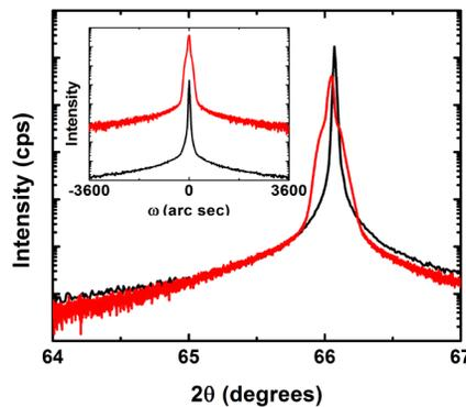
**Figure 26:**  $2\theta$  XRD curve for showing the (004) reflection for an In<sub>1-x</sub>Ga<sub>x</sub>P film (red curve) which is nearly lattice-matched to the GaAs substrate (black curve). Inset: Rocking curves for the film and substrate (004) peaks.
