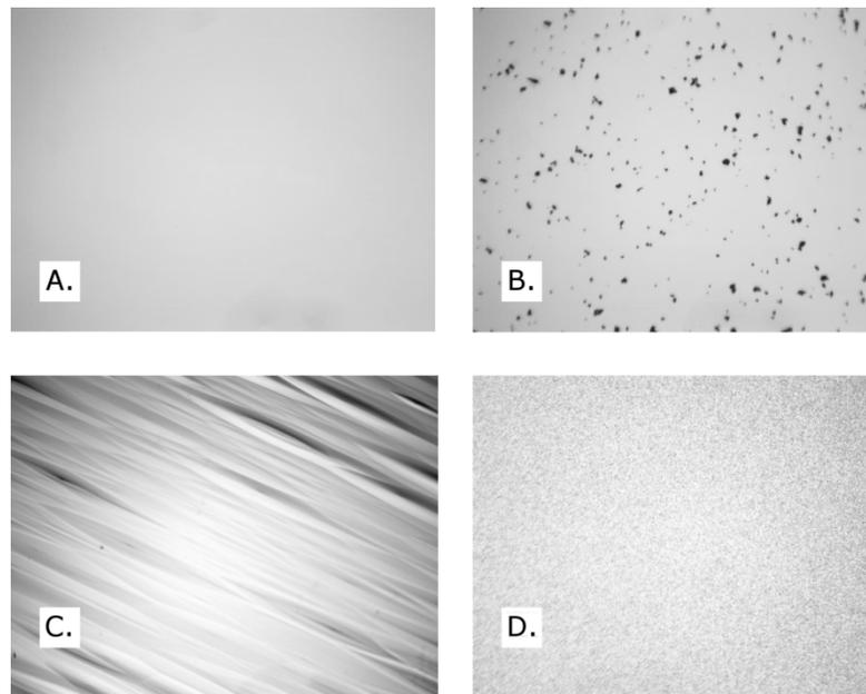
**Figure 9:** Optical microscope images of **A)** clean wafer surface **B)** surface after deposition of film from a powder source showing large density of surface defects **C)** surface after deposition from a highly Te-doped pellet showing elongated oval hillock defects **D)** rough surface after deposition from a wafer source.
