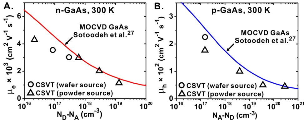
**Figure 3:** Hall mobilities of  $n$ - and  $p$ -GaAs films as a function of  $N_D$  and  $N_A$ . Solid curves represent the Hall mobility of high-quality epitaxially-grown MOCVD GaAs.<sup>48</sup>
