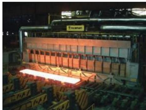
*A walking beam furnace for metal reheating*
