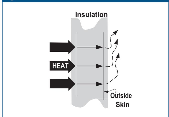
Figure 3. Radiation loss from heated to colder surface.
