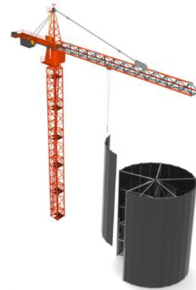
Figure 47. Rendering of modular receiver construction.
