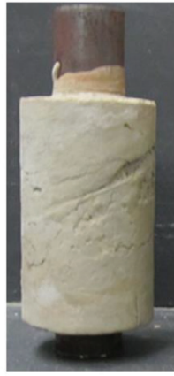
New BNL cement After 7 thermal shock cycles
