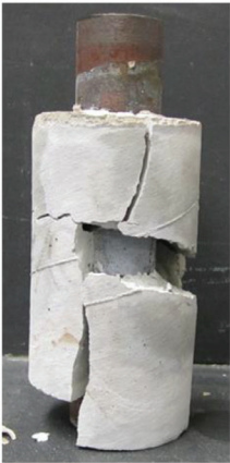
Conventional cement After 1 thermal shock cycle
