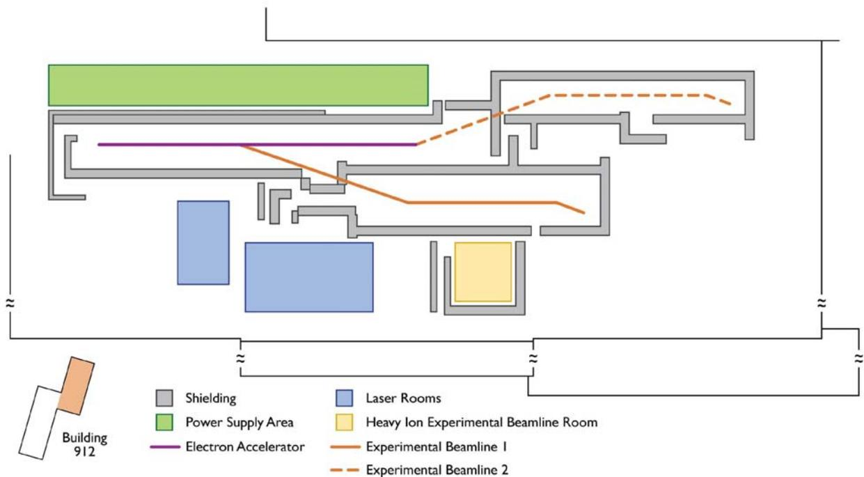
**Figure 5 Plan View of ATF Upgrade to 10 GeV in**
