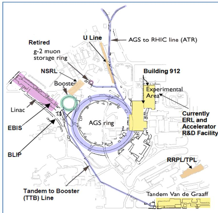
**Figure 4 AGS Complex that is Part of the C-AD Accelerator Complex**
