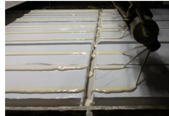
MAI-HD board fed through foaming line
