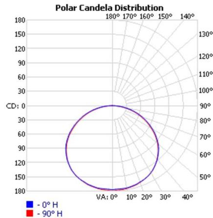
**Figure 11.** Polar plot of the photometric distribution from an eight-panel straight assembly of the Acuity Trilia™ OLED lighting system. The blue and red lines represent the 0° and 90° measurement planes, and are nearly identical. (Source: Acuity Brands’ Winona® Lighting, Test Report LTL25137.)
