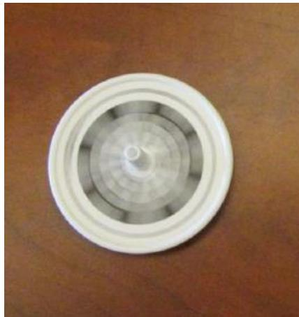
**Figure 9.** Flicker top showing “spokes” that indicate some level of flicker (stroboscopic effect) from the OLED and driver system dimmed with the 0-10 V dimmer. (Photo: Leslie North.)
