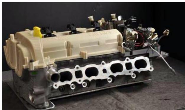
**FIGURE 5.** Modified cylinder head for the flexible ORNL engine platform to investigate in-cylinder reforming.
