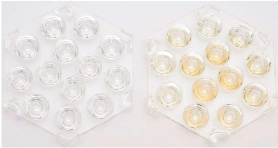
Figure 19. Lenses taken from two samples of model 12-96. The lens on the left is from the lamp model that failed catastrophically after 2,059 hours of continuous operation at 45°C. The lens on the right is from a lamp model that survived the entire test (13,925 hours) and showed significant discoloration due to excessive heat. The discoloration is especially pronounced in the center of the lens.
