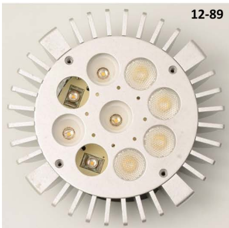
Figure 1. An example of an LED PAR38 lamp using individual secondary lenses.
