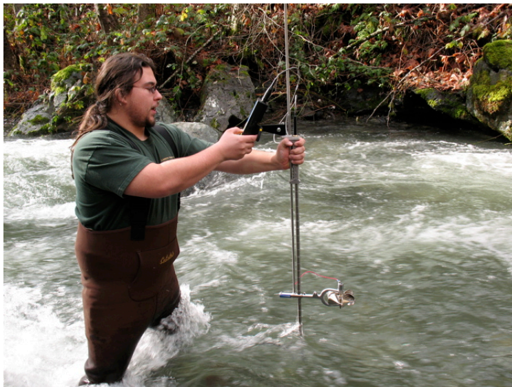
Figure 8: Yurok Tribe planner Austin Nova measures stream flow in Ke’Pel Creek
