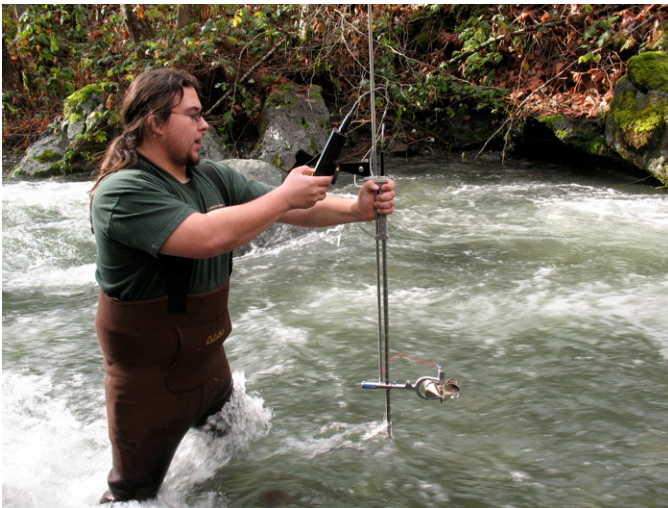
In-stream flow measurement.
