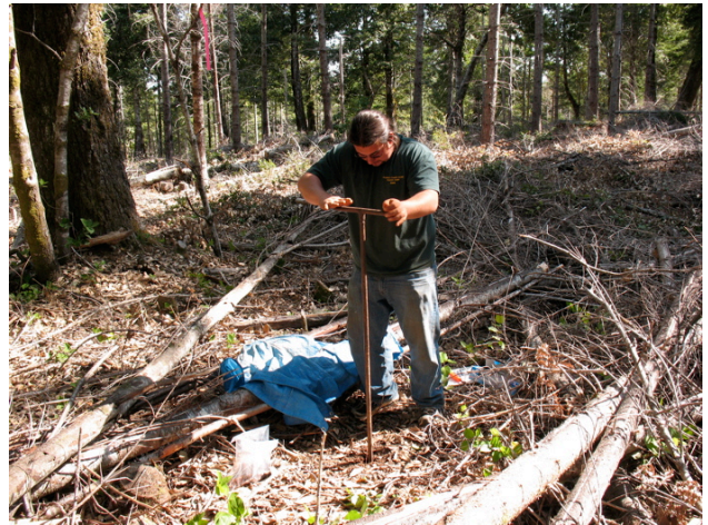
Taking soil samples for anchors.
