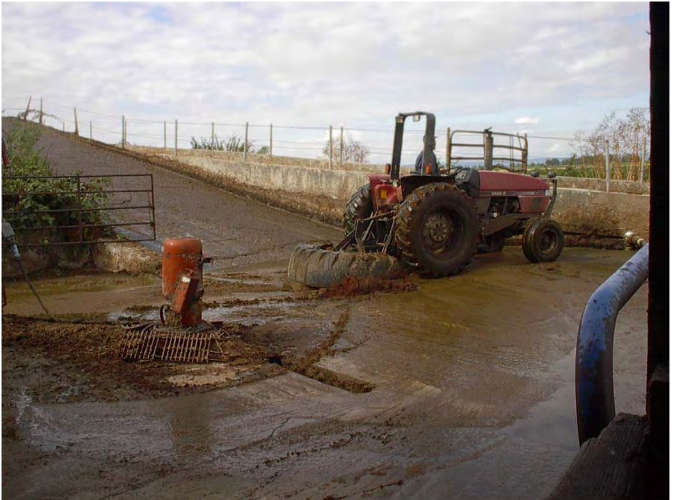
Figure 4. Typical Rubber Tire Scraped Manure Collection
