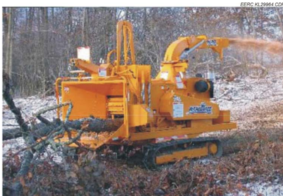
Figure 4. Wood chip production using a portable diesel grinder.
