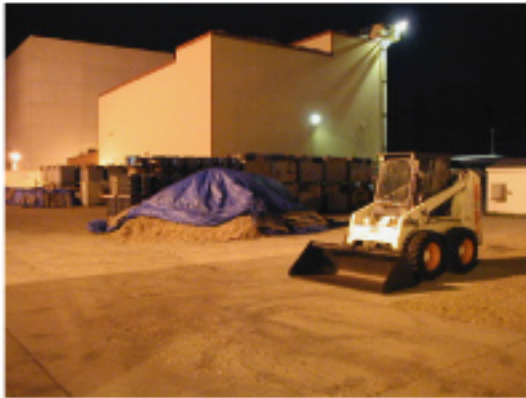
Chips were kept under a tarp and handled with a skid steer loader (Bobcat)
