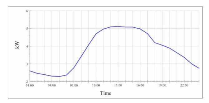
Figure 1 Load curve for typical day of commercial load on the Makah
