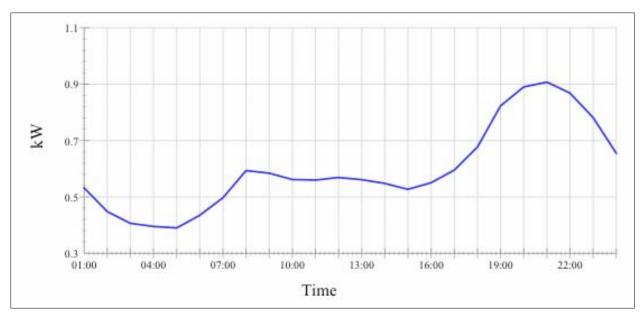
Figure 2 Load profile for typical day of residential load on the Makah
