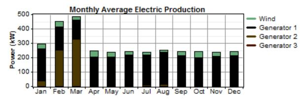
Figure 12 - Case "A" - Monthly generation from 100kW wind turbine
