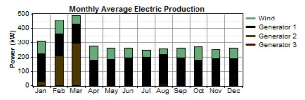
Figure 13 - Case "B" - Monthly generation from 225kW wind turbine
