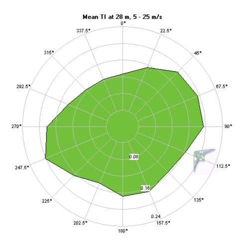
Figure 9 - Mean turbulence Intensity at 5-25m/s wind speed
