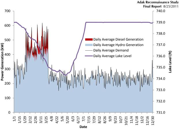
**Figure 5 – Option 10 (Lake Bonnie Rose to Mitt Lake) Performance Chart** The table below shows the energy distribution with the hydroelectric project as part of the generation system and the estimated annual fuel savings.
