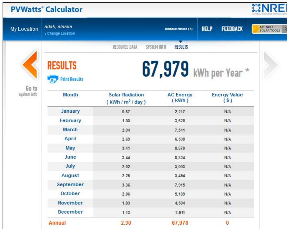
Figure 10. PVWatts solar resource estimate tool for a 100-kW PV system in Adak, Alaska
