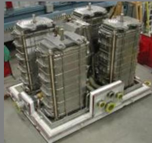
Four-Stack Module 1.4 megawatts
