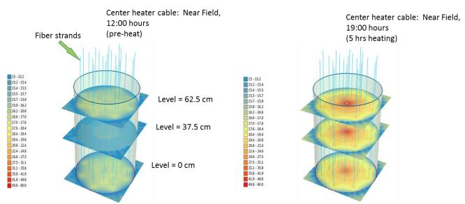
Figure 36. Data Acquired using the Fiber-Optic System prior to and after Heating for 5 hours.
