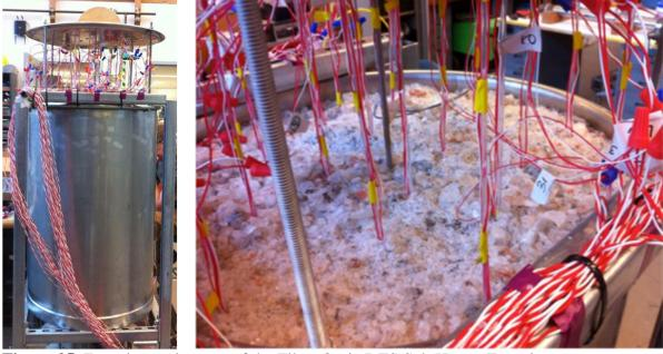
Figure 35. Experimental set-up of the Fiber-Optic DTS Salt Heater Experiments.
