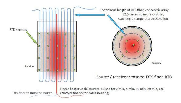
Figure 34. Schematic of the Batch Can Fiber-Optic Salt Test
