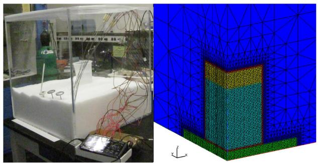
**Figure 22**. a) LANL equipment for laboratory investigations of granular salt under ambient and heated conditions. (b) Computational mesh for coupled THC simulations of these experiments.
