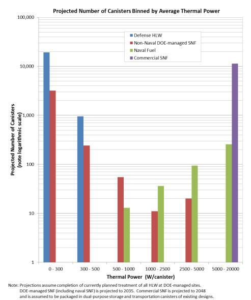
**Figure 2**. Number of Projected SNF and DHLW Canisters Binned by Average Thermal Power (from DOE, 2014, Figure 3; data sources: Carter and Leduc, 2013; SNL, 2014).
