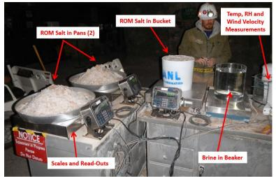
Figure 24. Brine and RoM Evaporation Experiments in WIPP.
