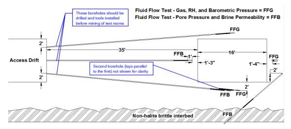
**Figure 14:** General layout of brine and gas testing borehole relative to the thermal test drifts. From Howard (2014).
