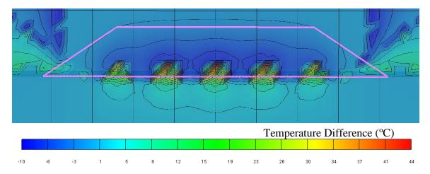
**Figure 19**. Temperature difference between a conduction-only and coupled TH simulation after 2 years (from Stauffer et al., 2012). This plot records the difference between the conduction-only temperature and the coupled TH temperature at each location. Red colors represent a higher (by as much as 44°C) temperature in the conduction-only model.
