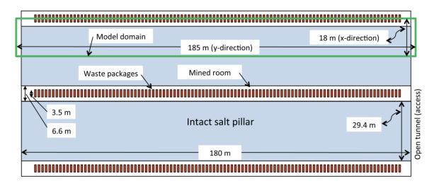
**Figure 15**. Plan view of repository heat transfer model for low-heat defense waste (from Harp et al., 2014).
