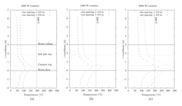
**Figure 18**. Steady state vertical temperature profiles for 1000W, 1500W, and 2000W canisters at 3 m and 6 m spacings (from Harp et al., 2014). Note: Temperatures far in excess of 200°C would probably not be considered in an actual design but are included here to illustrate the sensitivity of maximum temperature to the combination of spacing and thermal load.
