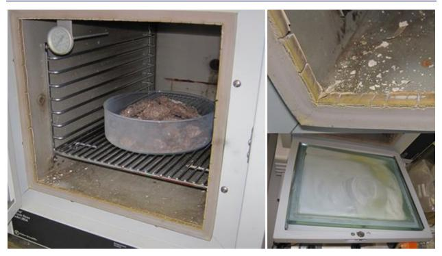
Figure 27. Oven Corrosion after Heating WIPP salt from Clay Seam F to 360 <sup>0</sup>C.
