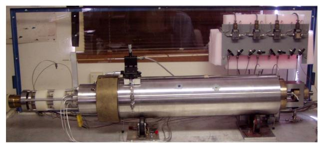
Figure 23. High Pressure and Temperature Vessel at LANL.
