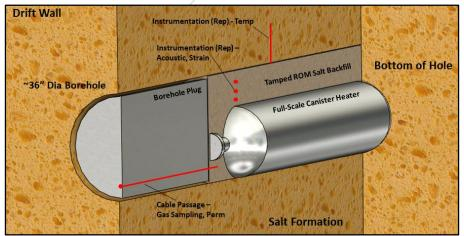
**Figure 4**. Schematic of the Borehole Emplacement Concept for this Test, including Representative Suggestions for Instrumentation.
