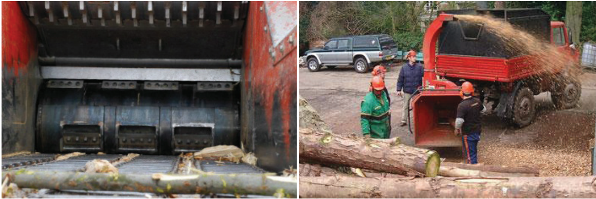
Figure 45. Potential wood chip production options. Horizontal chipper (left) and portable chipper (right).
