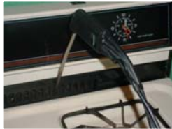
Insert the probe of the analyzer into the oven vent and read the CO content after the oven has warmed.
