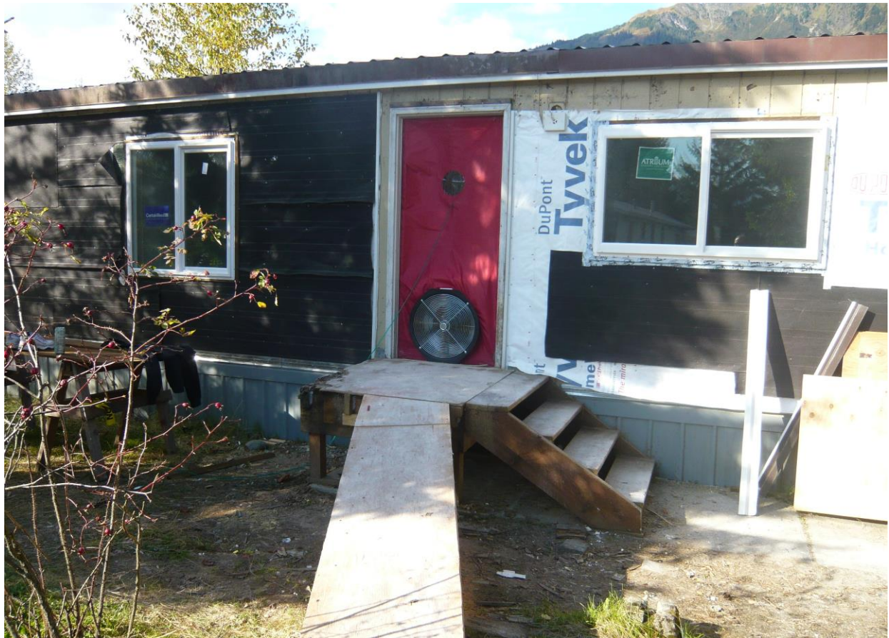
Example of Blower Door for instructional hands on diagnostics testing and training.
