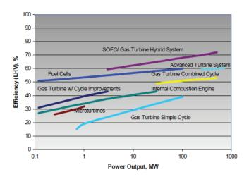
Figure 4.Q.3 summarizes efficiency trends as a function of power output for SOFC systems, including hybrid systems. At over 70% lower heating value (LHV) efficiency, the hybrid system would be more efficient than the combined cycle natural gas power plants powering the grid. Besides efficiency, there are other attributes that need to be considered (e.g., suitability for a desired operating strategy such as load following [see Table 4.Q.2]).
