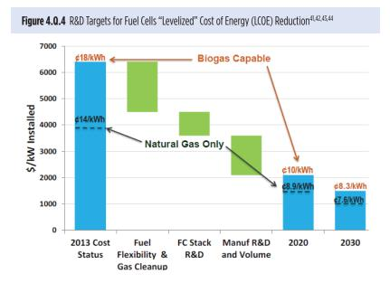
Figure 4.Q.4 shows the R&D waterfalls chart for CHP fuel cells on natural gas and biogas.
