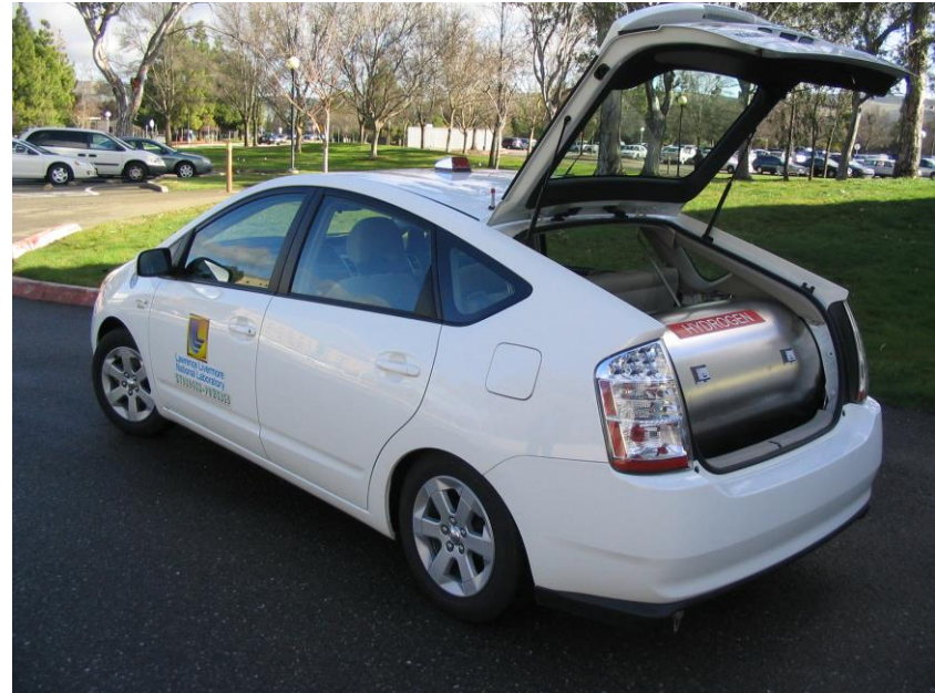
LLNL 350 bar cryogenic pressure vessel stores 10 kg LH 2 onboard a 2005 Prius
