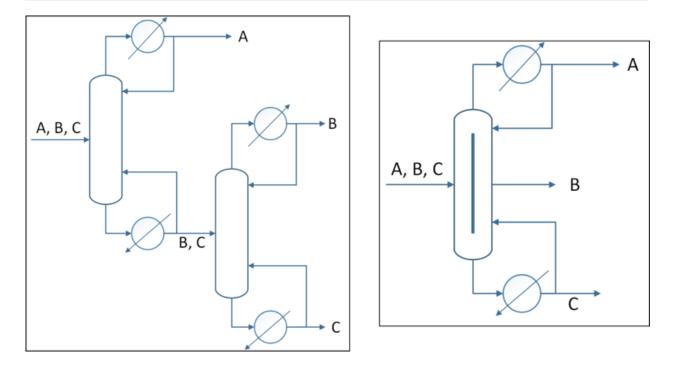
Figure 6.J.2 Distillation Column Configurations for Separating 3 Components (Left—Conventional Two-Column Configuration; Right—Divided Wall Column)
