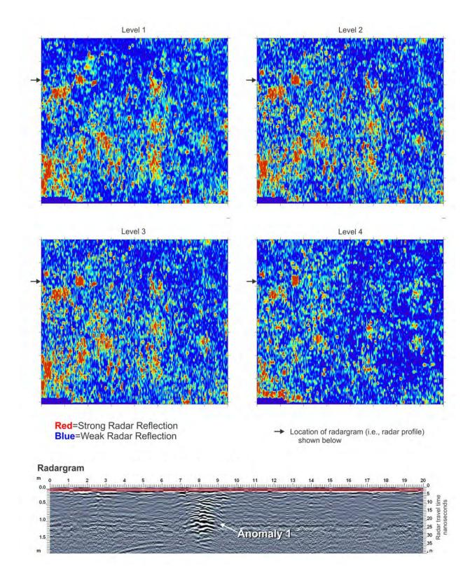
Figure 10.3. A selection of radar amplitude slice maps and an example radargram.
