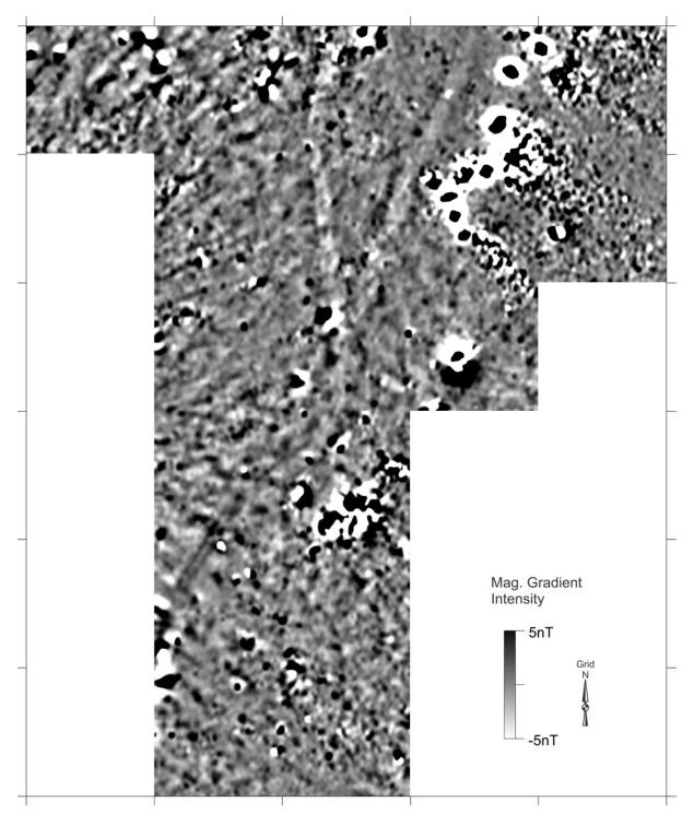
Figure 7.2. Magnetic gradient survey results at 33Pk348.
