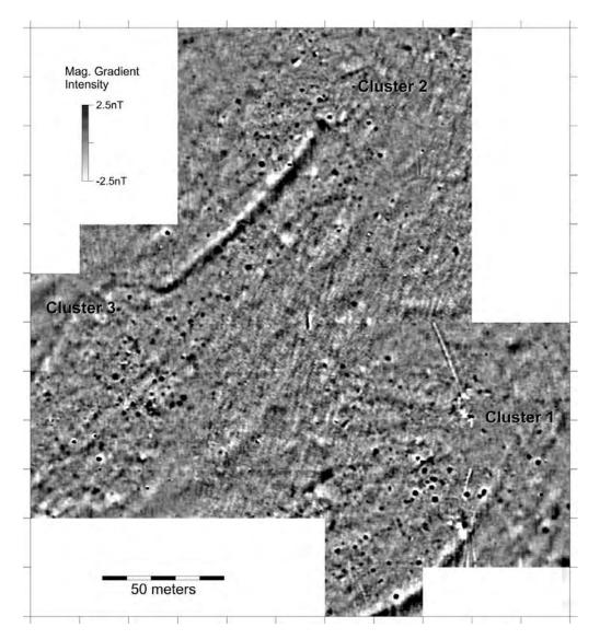
Figure 5.3. Example of magnetic gradient data from prehistoric Native American site, in this case the Brown's Bottom cluster of sites in Ross County, Ohio. Many of the small dark anomalies are archaeological features (see Pacheco et al. 2005, 2009a, 2009b for more on Brown's Bottom).
