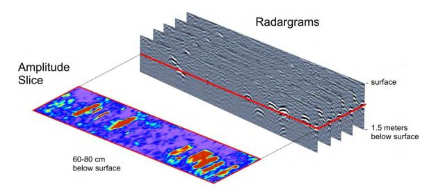
Figure 5.6. Creating amplitude slices from radargrams.
