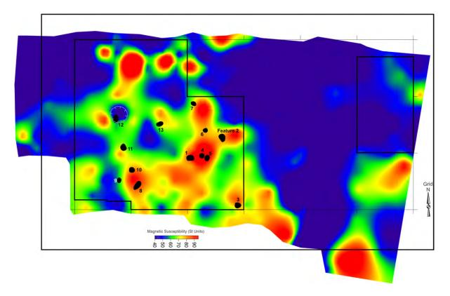
Figure 9.3. Magnetic gradient anomalies and magnetic susceptibility survey results.
