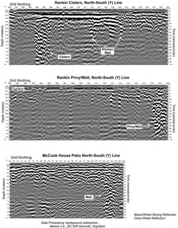
Figure 5.5. Radar profile examples with wells and cisterns from sites in Brown and Carroll Counties, Ohio.
