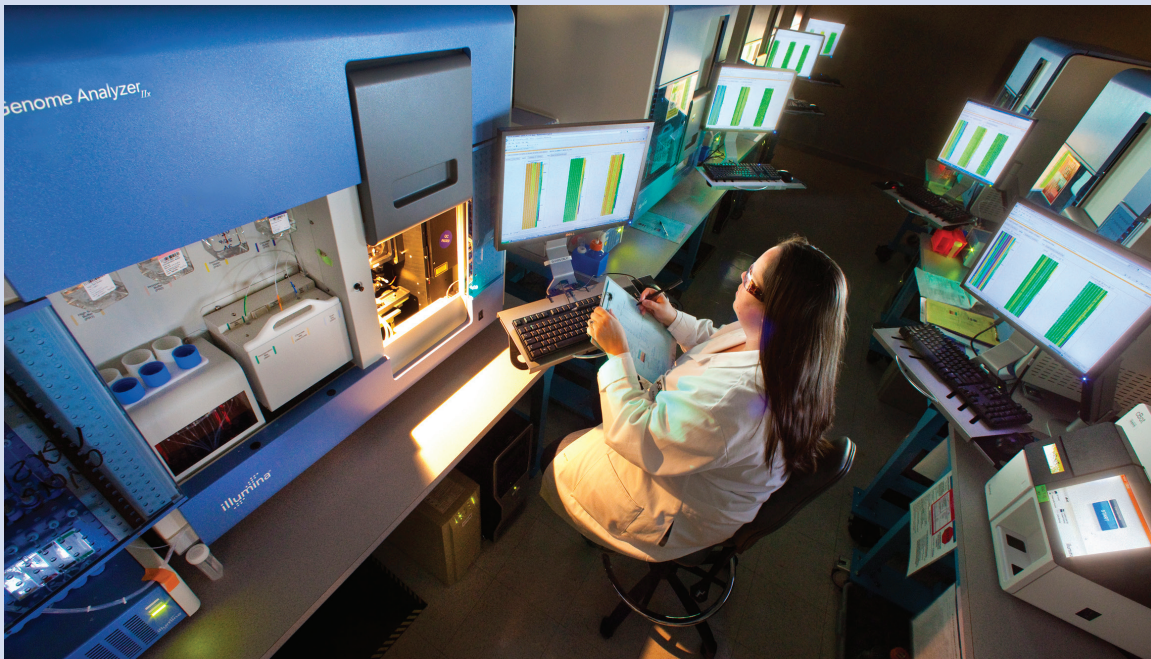
The Illumina sequencing platform, which has been incorporated in the DOE Joint Genome Institute's production line since 2008, allows for real-time detection during the sequencing-by-synthesis process. Genomic analysis and finishing efforts provide insight into the nature of infectious disease, the development of advanced therapeutics, and treatment approaches based on our increased understanding of disease mechanisms. Photo credit: LBNL, Roy Kaltschmidt, photographer
