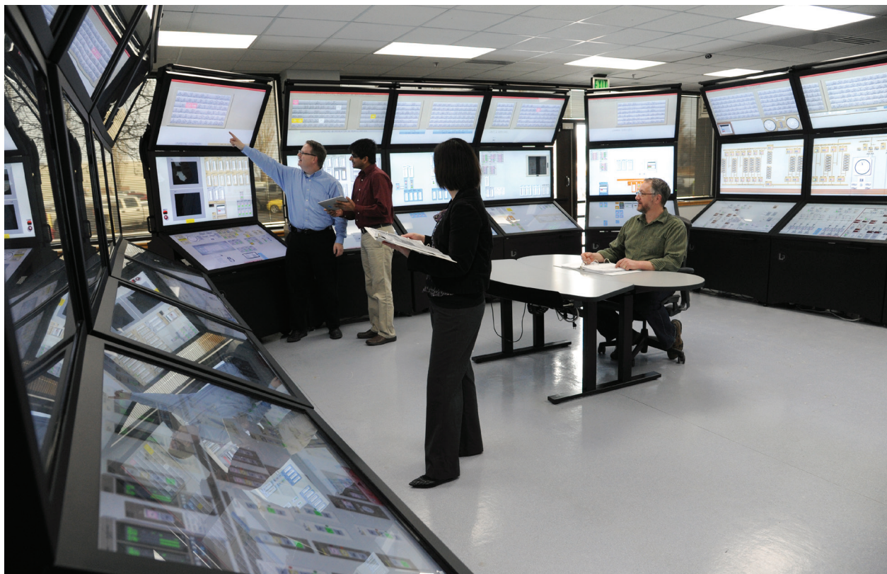
Serving as a virtual nuclear control room, the Human Systems Simulation Laboratory at INL supports modernization of instrumentation and control systems by providing an operating model to safely test new technologies before they are implemented in real commercial reactor control rooms. Photo credit: INL
