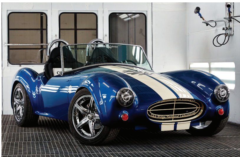
This 3D printed Shelby Cobra was printed at DOE's Manufacturing Demonstration Facility at ORNL and will allow research and development of integrated components to be tested and enhanced in real time, improving the use of sustainable, digital manufacturing solutions in the automotive industry. Photo credit: ORNL
