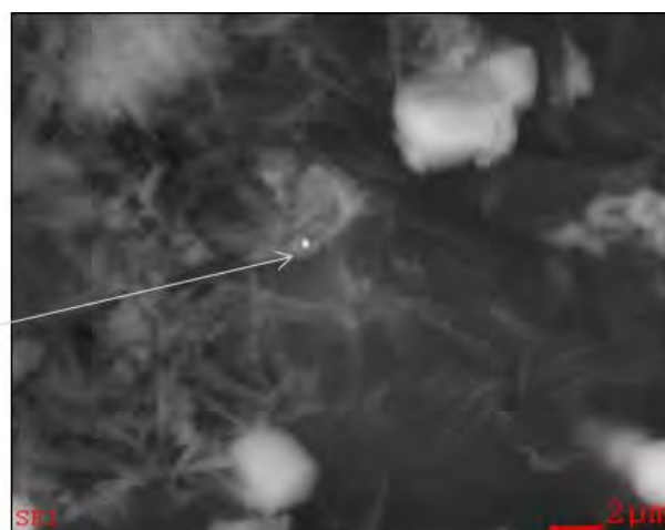
Figure C-10. SEM-EDS of small Pu particle associated with hairy salt particle from R16 C4
