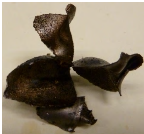
Figure G-6. ARC Bomb after 7 g 7-day dried 3.5 M HNO 3 / Swheat Scoop® Experiment
