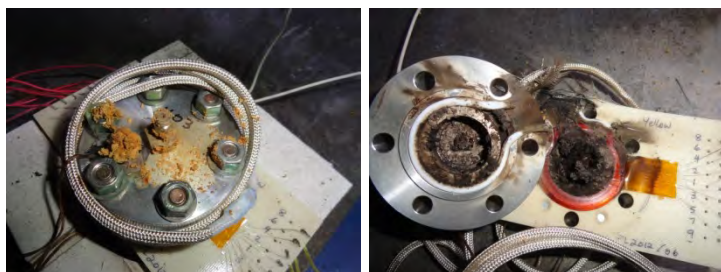
Figure G-26. Post-test images from Exp403. The left image shows that a substantial amount of material was expelled through the vent. The right image shows that the O-ring failed.
