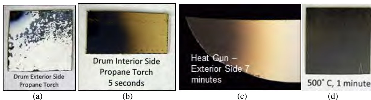
Figure D-32. Results of heating using a propane torch and heat gun.
