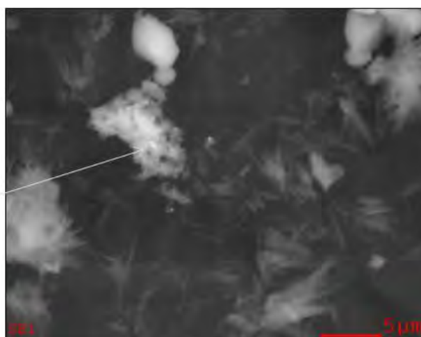
Figure C-11. SEM-EDS of a small particle of Pb associated with the hairy salt particle from R16 C4
