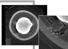
X-ray tomography to nondestructively locate defects/fractures
