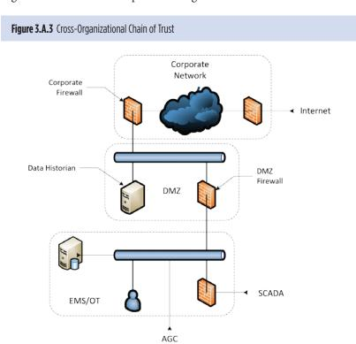
Key: SCADA = Supervisory Control and Data Acquisitions; EMS = Energy Management System; AGC = Automatic Governor Control.
