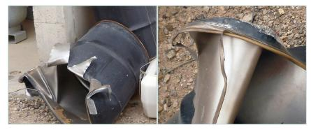
Figure 1-1. Views of exploded drum. The left image and the close-up image on the cover show the bottom of the exploded drum. The right image is a close-up view of the bottom seam of the drum.
