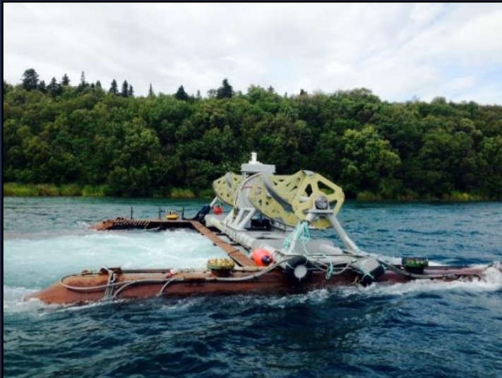
ORPC RivGen turbine in the Kvichak River
