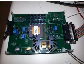
Figure - Board with radiation-hardened analog array.
