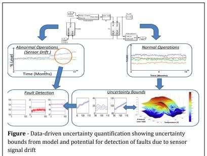
instrumented flow loop showed the ability to compute UQ bounds from measured data, as well as potential insights into the development of fault detection techniques for OLM sensor fault identification and localization. Results also indicated that the UQ method can track changes in the uncertainty bounds as operating conditions change.
