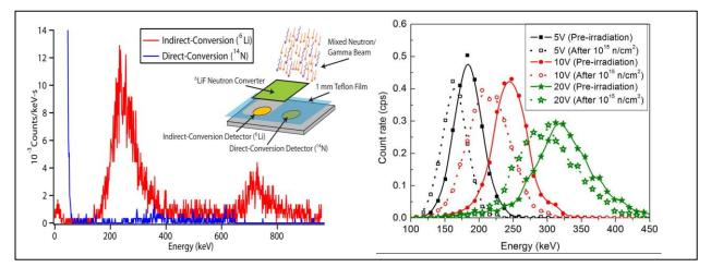
**Figure** - (left) Red curve shows the detected neutron signal in a high flux neutron beam, blue curve shows the fast neutron response; (right) shows the still functioning sensors after in-core irradiation at OSU Research Reactor.
