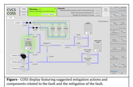
events and return the plant to a safe operating condition with minimal deviation. The system under development operates as a multi-stage process that sequentially aids the operator in the remediation and resolution of an upset event. The overall technique involves six distinct stages: validation, detection, diagnosis, mitigation, monitoring (for successful mitigation), and recovery (to pre-fault plant conditions).
