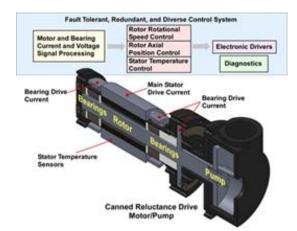
Figure - Fault-tolerant, redundant, and diverse control embedded in coolant circulation pump
