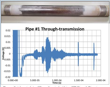
Figure - Stainless steel pipe (25 mm diameter) with two PZT/Bismuth Titanate sprayon comb transducers (with 4-1.6 mm wide elements) generates axisymmetric L(0,n)modes when excited at 1.83 MHz.
