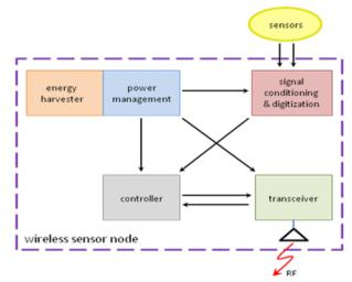
Figure - Elements of a self-powered wireless sensor node.
