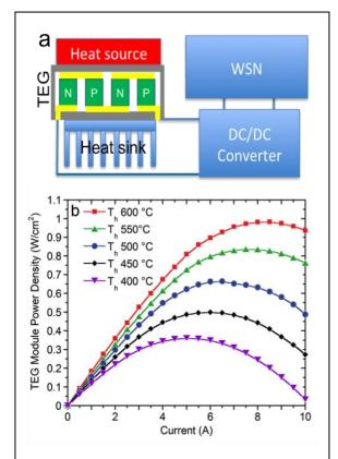
**Figure** - (a) Schematic of self-powered wireless sensor node (WSN) using thermoelectric generator (TEG) (b) Electric power density vs. current for various hot-side temperature of nanobulk half-Heusler TEGs.
