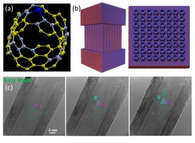
**Fig. 1** - (a) DFT simulation of BC<sub>4</sub>N nanotube with Li. (b) MD model of BNNTs for simulating displacement cascade. An 8×8 array of BNNTs is sandwiched by two cubic boron nitride substrates. (c) Early-stage evolution of irradiation-induced vacancy defects in multi-walled BNNTs as observed through in-situ TEM.
