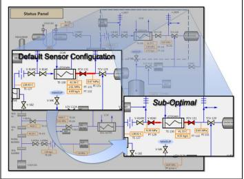
**Figure** - The Spatial Localization of a Fault is Sensitive to the Sensor Set Including Details such as the Number and Types of Sensors
