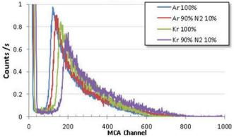
Figure 2 - Measured effects of admixture of nitrogen into a noble fill gas on the amplitude of pulses due to fission
