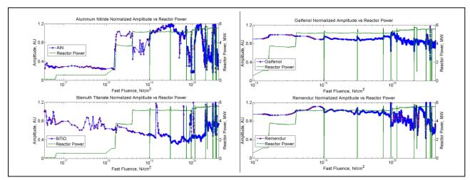
**Figure** - Signal amplitude of transducers as a function of total fluence. Bismuth Titanate transducer has degraded, as expected. Other transducers continue to operate with minimal radiation induced degradation.
