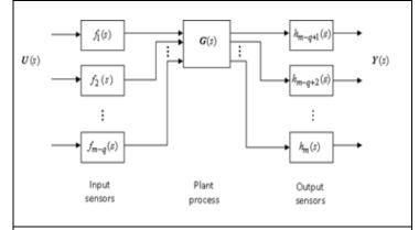
**Figure** - General form of process amenable to treatment. Typically each sensor is represented by a first order lag. Measured inputs and outputs are shown.
