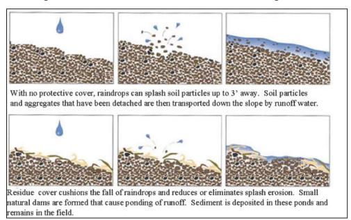
Figure 3.4-3: Effects of Ground Cover on Reducing Erosion
