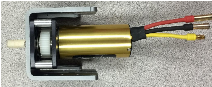
Figure 10. ElectriFly Gearbox Attached to ElectriFly Generator
