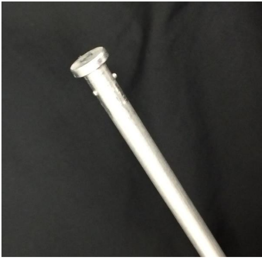
Figure 2. Connecting Rod with Pinned Plug
