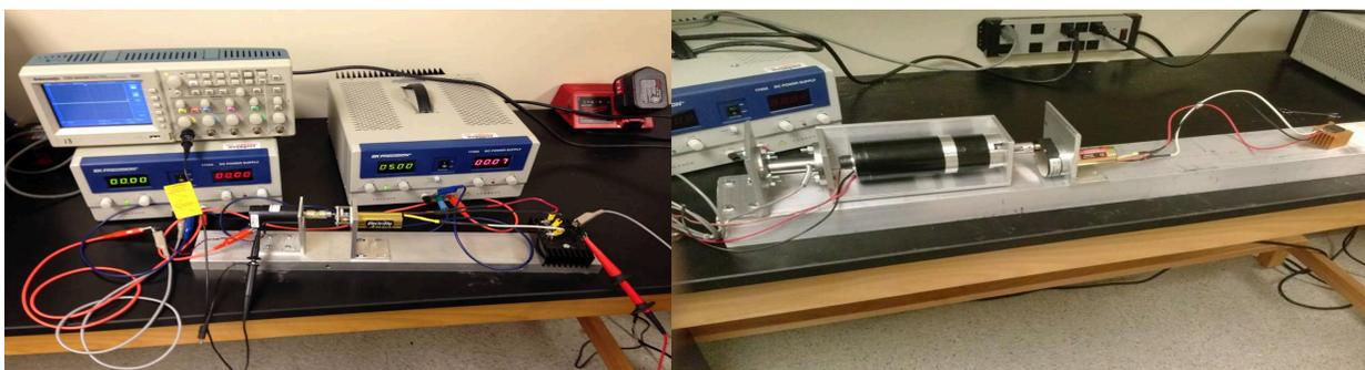
Figure 2. The earliest testing rig (left) and the torque cell rig (right).
