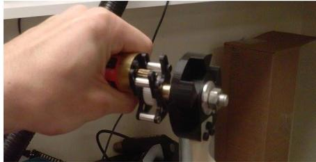
*Figure 4. An example of gearbox tested with the torque cell rig. The gearbox ratio was 4.5:1.*
