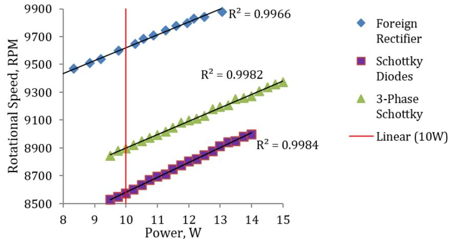
Figure 1. RPM vs. Power for three rectifying systems.
