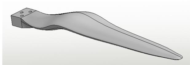
*Figure 10. The S818 style blade used in the most recent prototype.*
