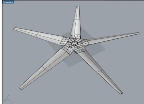
*Figure 8. Blade and hub iteration assembled in CAD.*
