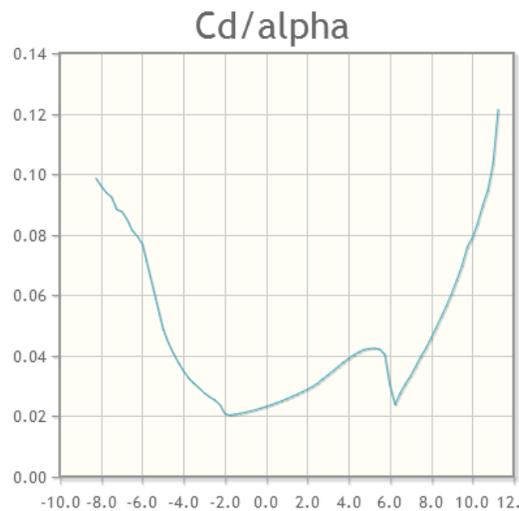
Figure 7. Example of drag coefficient vs angle of attack graph for the 6 Series airfoil.
