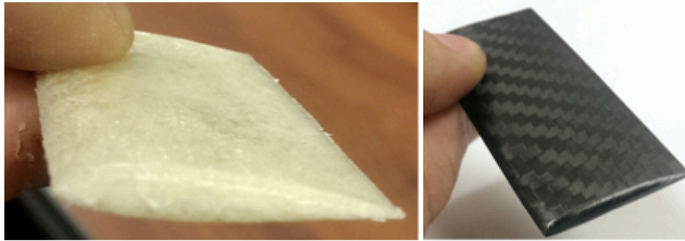
Figure 6 - Blade core (left) and skinned blade
